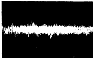
Focusing signal P108 Pin2 V:10mV/div. H:0.5ms/div.
